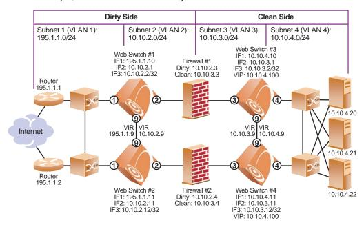
Figure 13-9 Four-Subnet FWLB Example Network
